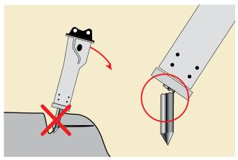
Try to avoid bending stresses on working tools at all times to avoid overstressing of the material.
