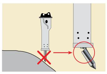
Working tools should always be positioned at right angles to the working surface to avoid long-term secondary damage.
