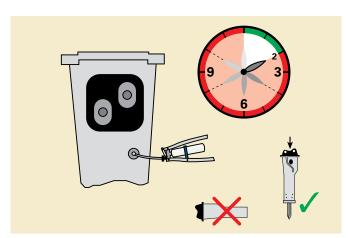
Lubricate working tools at regular intervals. When lubricating, observe the correct position to avoid over-greasing.
